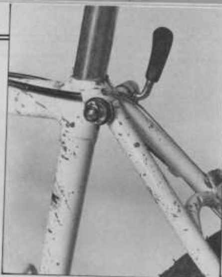
Rear brake: No chintzy cable guides for the Hammer. Park Pre used a special casting that doubles as a seat tube reinforcer, fast-back seat stay mount and built-in rear brake cable guide.
